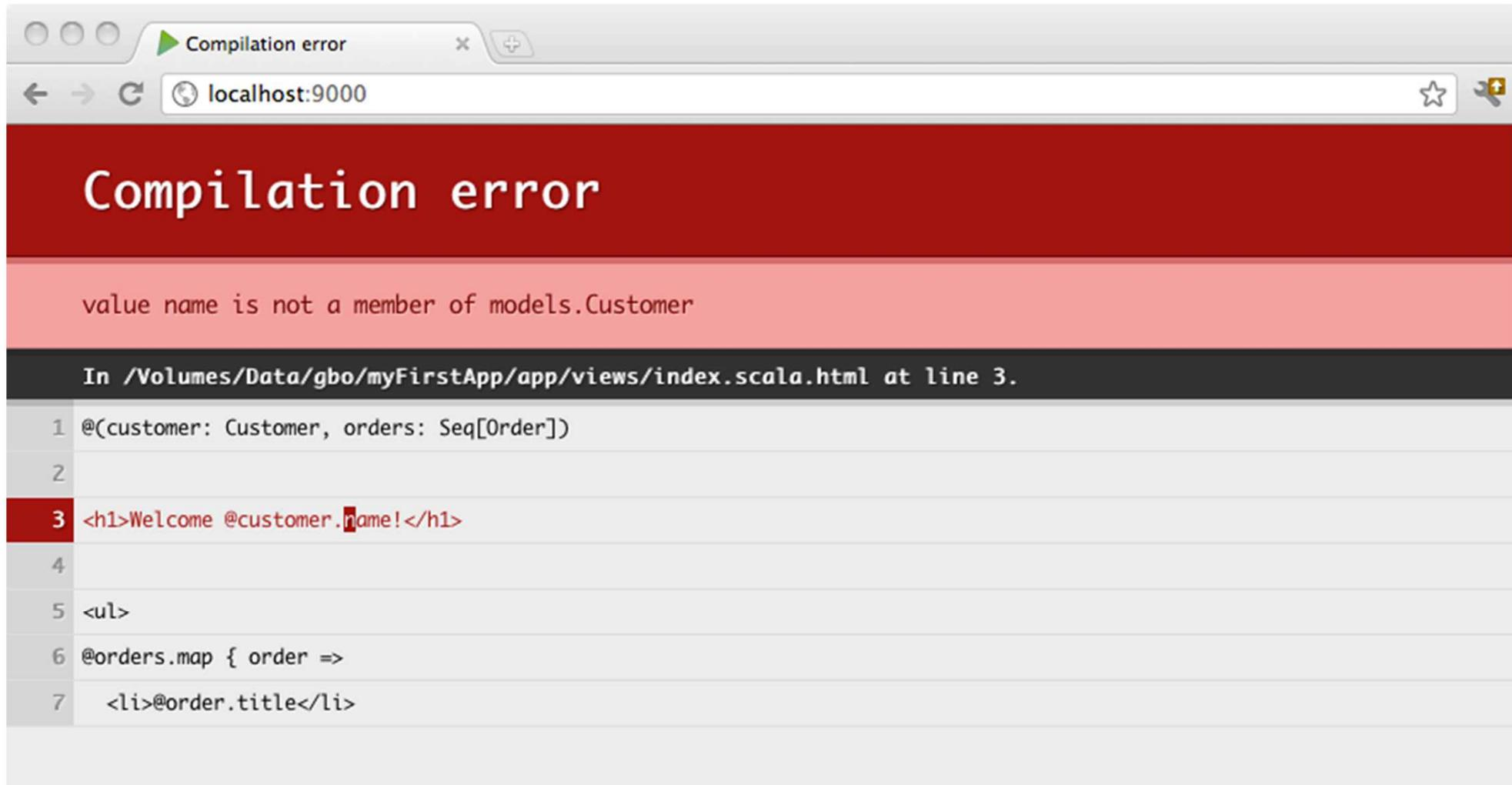
A screenshot of a web browser window titled "Compilation error". The address bar shows "localhost:9000". The main content area has a red header with the text "Compilation error". Below the header, a pink section displays the error message: "value name is not a member of models.Customer". A dark grey section below the error message shows the file path: "In /Volumes/Data/gbo/myFirstApp/app/views/index.scala.html at line 3.". The code editor shows the following Scala code:
