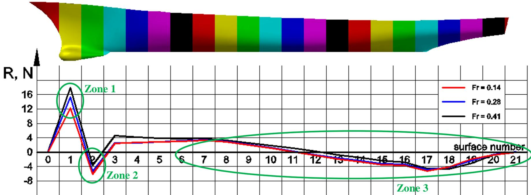
Zone 1: Maximum peak of resistance force on the nose part of the bulb;
