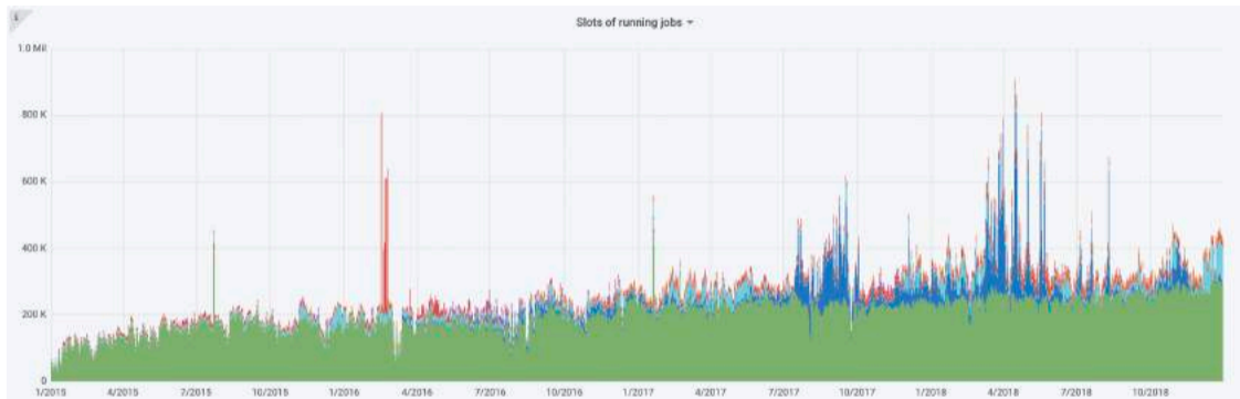
Figure 2 – Number of running CPU core slots grouped by resource type: GRID sites, HPC with closed network infrastructure, Clouds, HPC with closed network infrastructure, BOINC - volunteered computing resources
